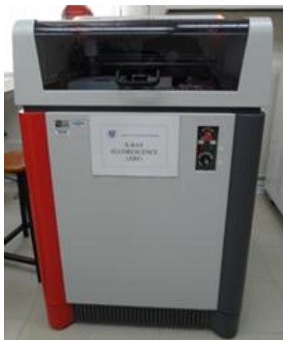
Figure 5 X-Ray Fluorescence (XRF)
