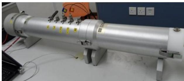
Figure 7 Impedance Tube
