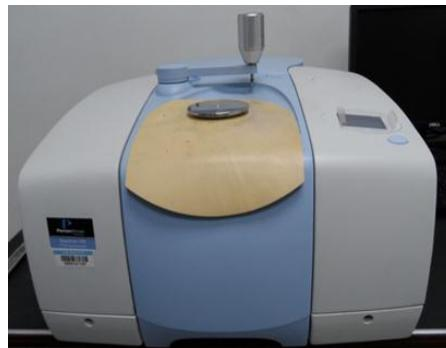
Figure 6 Fourier Transform Infra-Red (FTIR)
