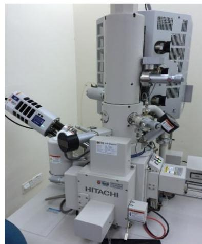
Figure 3 Field Emission Scanning Electron Microscopy (FESEM)
