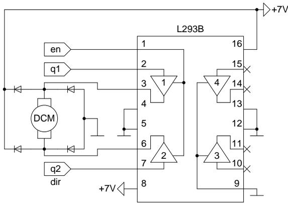
Figure 9 Power electronic circuit. The transistors at the output of the bridge are bipolar
