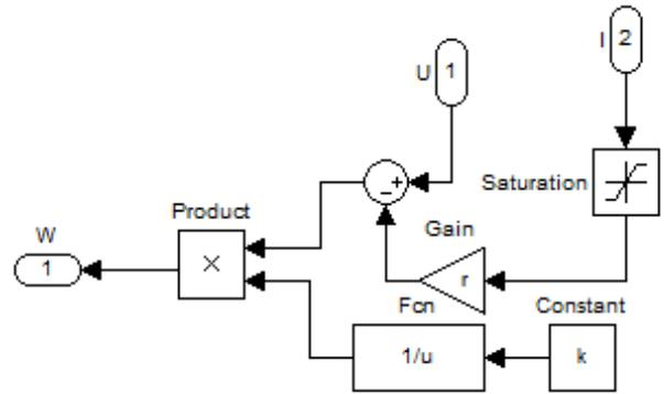
Figure 5 The Matlab Simulink model of the speed estimator device
