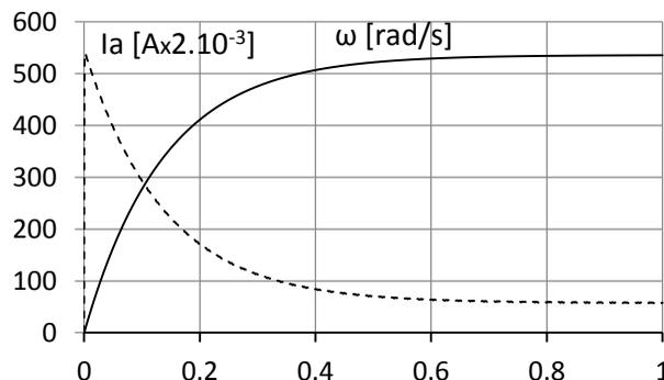
Figure 2 Starting Motor transition process.  $U_z=12V$ ,  $I_c=116mA$ ;  $W_{MAX}=534rad/s$ .
