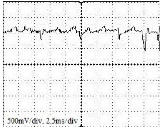
Figure 14 High motor speed anchor current. The variations of the anchor current are smaller in high speed.
