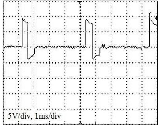
Figure 13 Power side soft chopping PWM. The upper spike corresponds to the upper bridge transistor saturation; the down spike reflects the down bridge transistor saturation.
