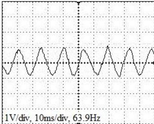
Figure 11 Lowest motor speed:  $f/4$  gives rot./s
