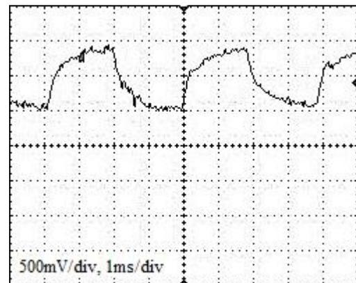
Figure 15 Low motor speed anchor current. Variations of the anchor current are bigger than in high speeds.
