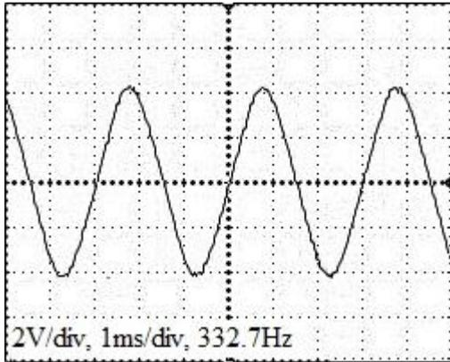
Figure 10 Highest motor speed:  $f/4$  gives rot./s
