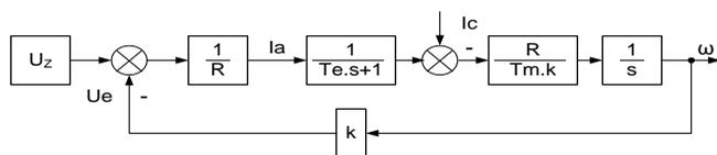
Figure 1 Direct Current Motor Matlab Simulink Model
