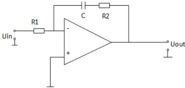
Figure 3 Analogue variant of the PI regulator
