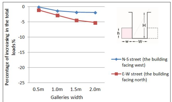
Figure 13 Total energy required to achieve comfort in the examined building as a result of varying the galleries width by IDA ICE.
