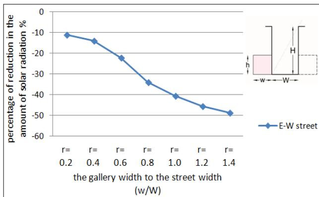
Figure 8 Incident solar radiation on (E-W) street as a result of varying the galleries width by ECOTECT
