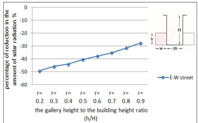
Figure 9 Incident solar radiation on (E-W) street as a result of varying the galleries height by ECOTECT
