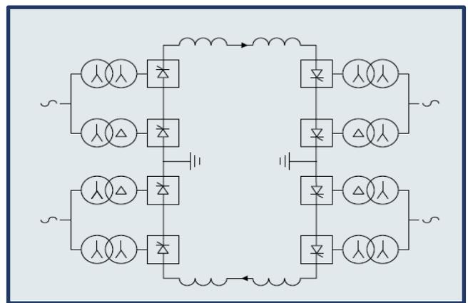
Figure (1): Bipolar HVDC System [3]
