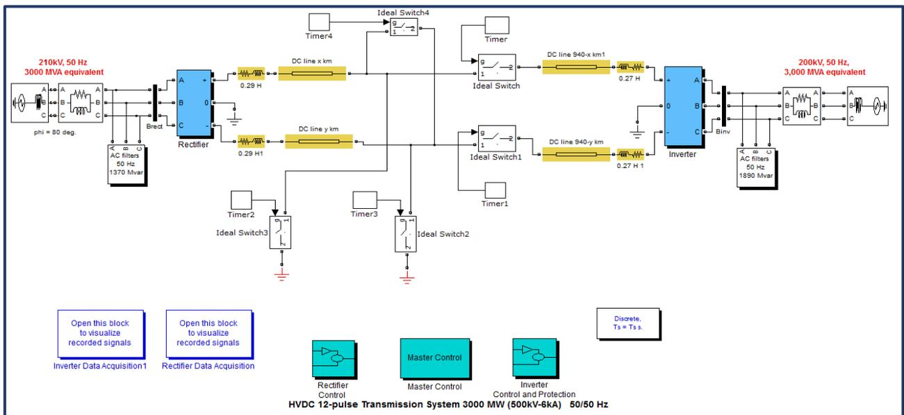
Figure (4): HVDC MATLAB Model
