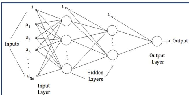
Figure (2): Basic 3 –Layer Feed-Forward NN [11]
